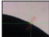
Digitise the cutting edge profile at the first position required
